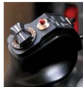
The aircraft's electric trim control is located on the yoke.
